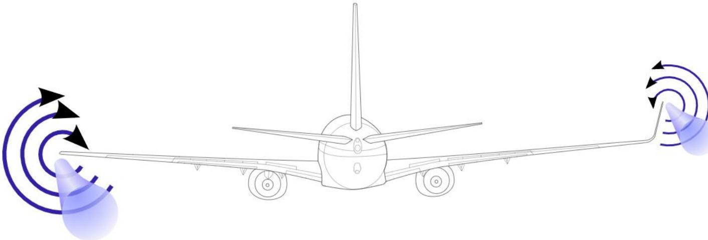
Longer wingspan | Winglets | Geared turbo fan engines
